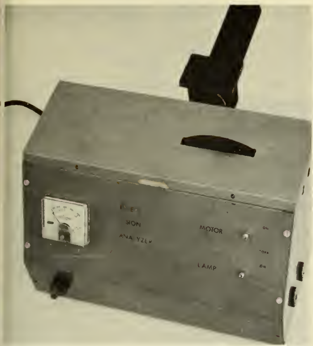
FIGURE 13.—External view of assembled vision analyzer with attached light-conduction tube and filter holder.
